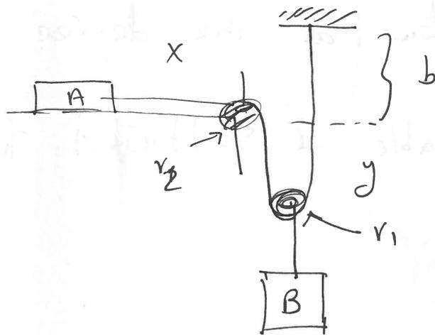
parameters are  $r_1, r_2, b$ . The constraint is that the total length of the cable
