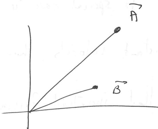
$\vec{r}_{A|B}$  is the position of A, as seen by B.
