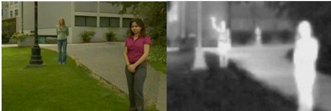
Figure 1. On a typical day, different amounts of heat are radiated from different objects in the same environment. The above pictures were taken with a normal camera (left) and an infrared camera (right) on a cool day in June. Objects emitting more radiation appear lighter and those emitting less radiation appear dark -- the people in this picture are much hotter than the environment and so stand out as being much lighter in colour in IR camera.
